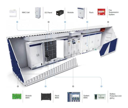
Figure 3 Indicative arrangement of containerised module
